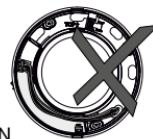
No 100–240 V cables may be laid over the electronics component (Figure N).
